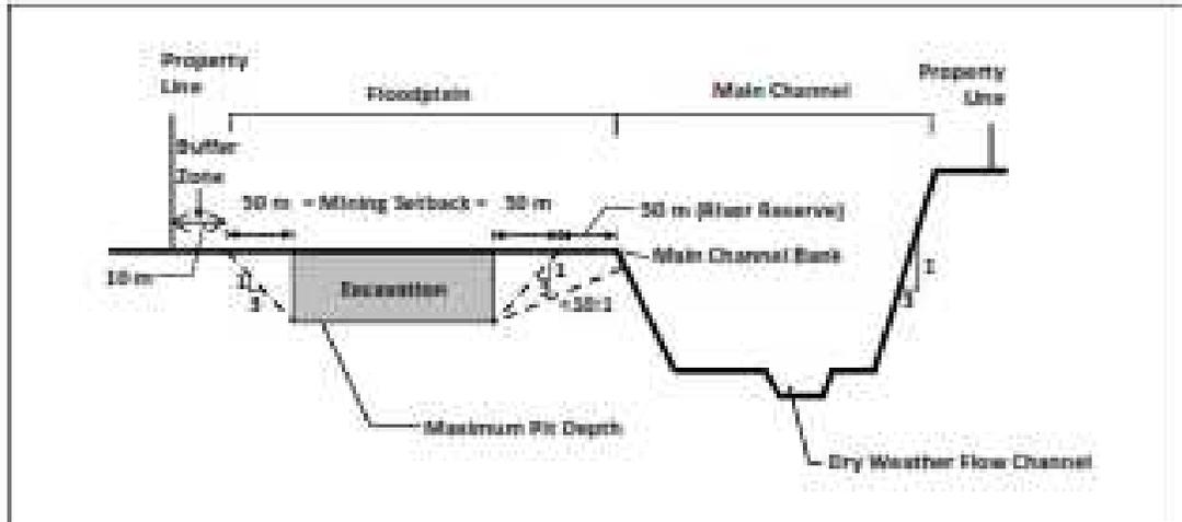
**Fig.10: Floodplain Excavation Pit Geometry for Streamlined Floodplain**
